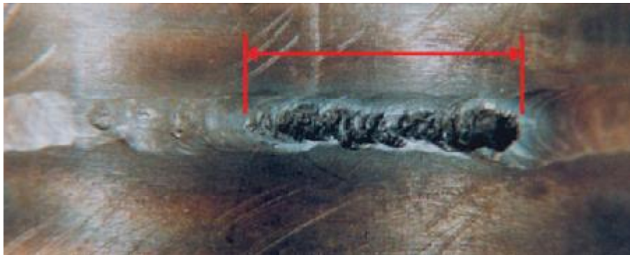
Figure 44—Surface Oxidation Due to Insufficient Shielding in a Gas Tungsten Arc Weld
