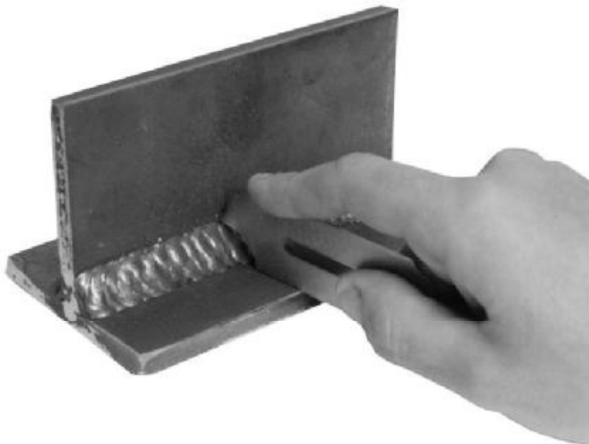
Figure 48—Evaluating a Convex Fillet Weld
