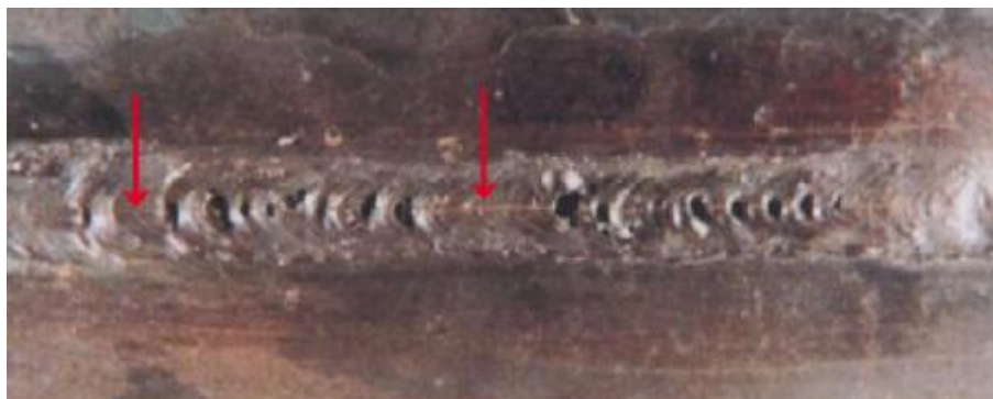
Figure 29—Longitudinal Crack and Aligned Porosity
