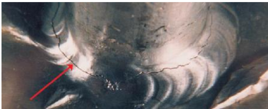
Figure 33—Longitudinal Cracks Propagating from Crater Crack
