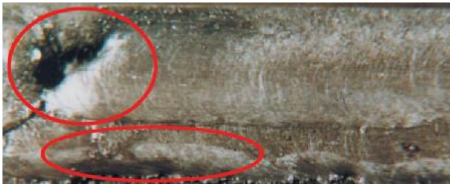
Figure 16—Incomplete Fusion Between the Weld and Base Metal
