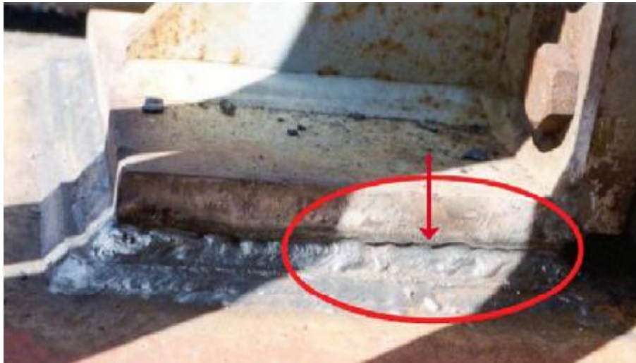
Figure 21—Undercut at Fillet Weld Toe
