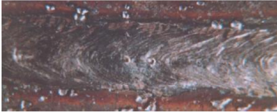
Figure 9—Surface Appearance of Piping Porosity
