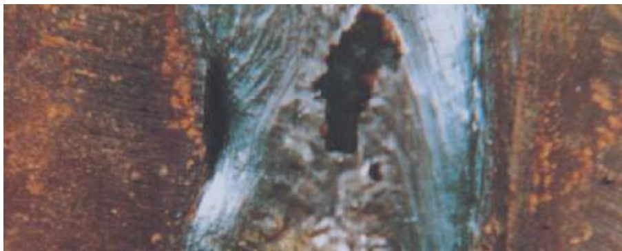
Figure 14—Incomplete Fusion at the Groove Face
