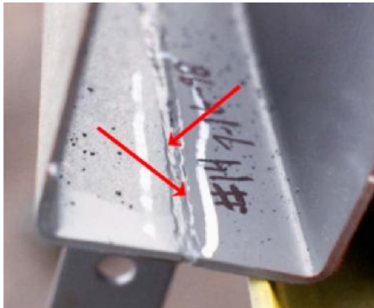
Figure 23—Underfill in a Groove Weld Made Using GMAW
