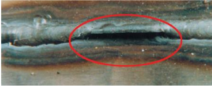
Figure 18—Incomplete Joint Penetration with Consumable Insert
