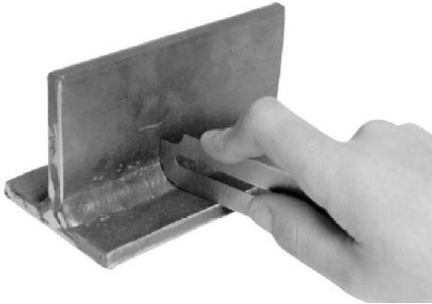
Figure 49—Evaluating a Concave Fillet Weld
