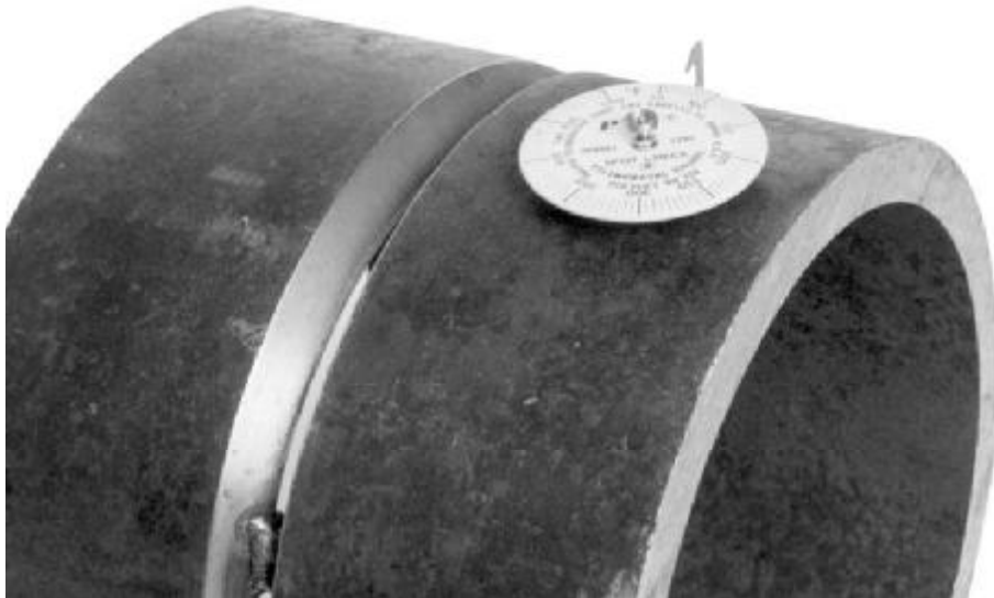
Figure 46—Surface Contact Thermometer
