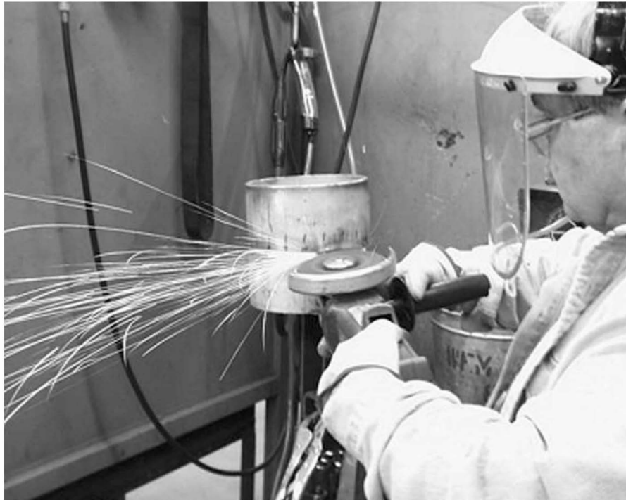
Figure 304-3.1-3 Grinding of Weld Flaw
